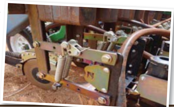
An increased number of springs enabled sufficient penetration for planting in stubble.
